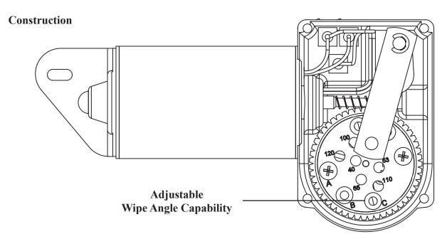
The WWF motor is set for a default 110° wipe angle that be adjusted at the time of installation to the angles shown. Quantity orders can be supplied set at 40°, 53°, 65°, 85°, 100° and 110°. Left or right hand park position is determined from view shown above and can be adjusted.
